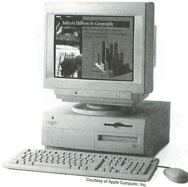
Figure 2.4 Power Macintosh 7200: a 75 or 90MHz 601 processor that can be upgraded to a 7500 motherboard.
